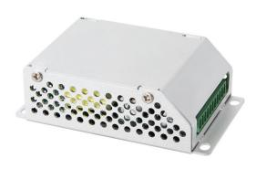
Dimensions (LxWxH):  $100.0 \times 60.0 \times 30.0$ mm (3.94 x 2.36 x 1.18 inch) 145g (0.32 lbs)
