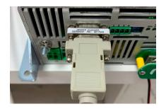
2.2 CONNECT THE SERIAL PORT WITH A NULL CABLE. PINS 2 AND 3 ARE CROSSED:
