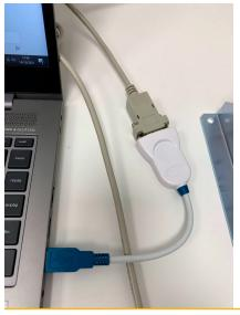
2.3 CONNECT THE SERIAL PORT TO THE COMPUTER USING A RS-232 TO USB ADAPTER:
