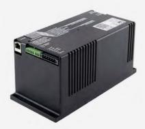
Power [W] 120 Input Voltage Range [V] 184 - 265 Output Voltage Range [V] 0 - 57.6 **Cooling:** Natural convection Dimensions [LxWxH in mm]: 247 x 115 x 115
