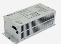
Power [W] 150 Input Voltage Range [V] 184 - 264 Output Voltage Range [V] 0 - 57.6 **Cooling:** Natural convection
