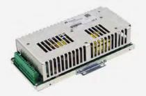
Power [W] 200 - 230 Input Voltage Range [V] ±20% Output Voltage Range [V] 12 - 57.6 **Cooling:** Natural convection Dimensions [LxWxH in mm]: 100 x 220 x 45
