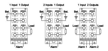
Use cables of adequate cross-section to connect inputs and outputs. The following table lists the maximum currents and the minimum cross-sections for the cables used for each connection in a complete equipment
