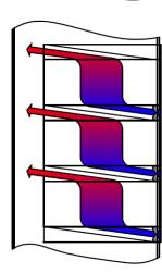
4 When the natural convection cooling is required, several CKR-2000 can also be stacked. To this it is necessary to leave a gap of 3U between them and include plates that conduct the hot air from the intermediate units to the rear side.
